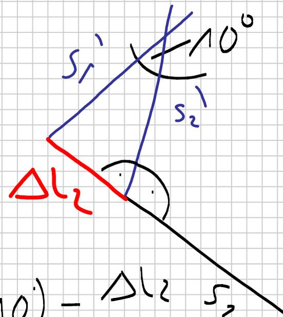
$$s_1' = \frac{\Delta L_2}{\sin(10^\circ)} = \frac{|-0,0107 \text{ mm}|}{\sin(10^\circ)} = 0,0616 \text{ mm}$$
